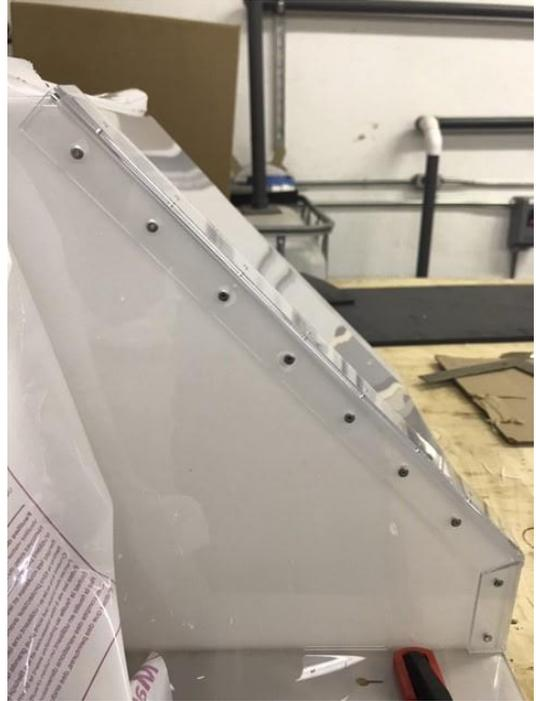
Figure 8 The attachments and cover attached with rivets
